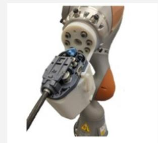
Custom housing that interfaces with da Vinci endoWrist tools and mounts onto the KUKA flange
