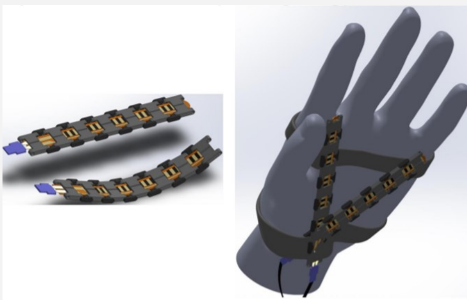
Flex sensor and modular 3D printed chain on the palm
